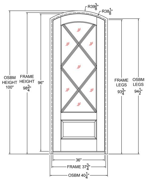
MAHOGANY 1-3/4" STAIN GRADE RO: 38-1/2" X 99-1/2" CLEAR BEVEL **GLASS** OTHER (CUSTOM): 4-9/16" 6-9/16" **JAMB SIZE** OTHER (CUSTOM): (2") 180 BRICKMOULD APPLIED LOOSE **EXT TRIM** (5/4 X 4) FLAT S4S EXT. TRIM (UPCHARGE APPLIES) APPLIED LOOSE ORB (BLACK) SATIN NICKEL HINGES OTHER: SILL BRONZE NICKEL [ DOUBLE BORE (5-1/2" O.C.) BACKSET: 2-3/8" LOCK **PREP** G-U MULTIPOINT LOCK SYSTEM (UPCHARGE APPLIES) RH I/S LH I/S **SWING** LH O/S RH O/S NOTES:
