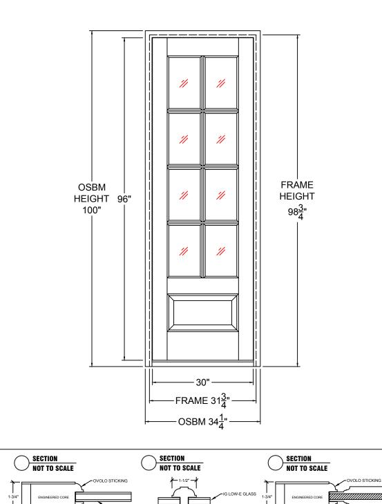
MAHOGANY 1-3/4" STAIN GRADE RO: 32-1/2" X 99-1/2" FLEMISH CLEAR BEVEL **GLASS** OTHER (CUSTOM): 4-9/16" 6-9/16" **JAMB SIZE** OTHER (CUSTOM): (2") 180 BRICKMOULD LOOSE APPLIED **EXT TRIM** (5/4 X 4) FLAT S4S EXT. TRIM (UPCHARGE APPLIES) APPLIED LOOSE ORB (BLACK) SATIN NICKEL HINGES OTHER: SILL BRONZE NICKEL [ DOUBLE BORE (5-1/2" O.C.) BACKSET: 2-3/8" LOCK **PREP** G-U MULTIPOINT LOCK SYSTEM (UPCHARGE APPLIES) RH I/S LH I/S **SWING** LH O/S RH O/S NOTES:
